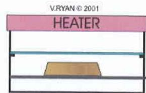
PLASTIC SHEET IS PLACED ABOVE THE MOULD AND CLAMPED SECURELY.
