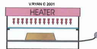
THE ELECTRIC HEATER IS TURNED ON TO WARM THE PLASTIC SHEET.
