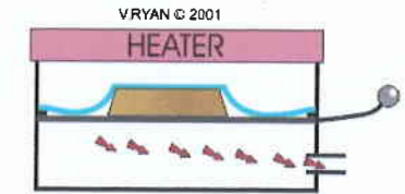
THE AIR IS PUMPED OUT OF THE AREA BELOW THE PLASTIC AND MOULD.
