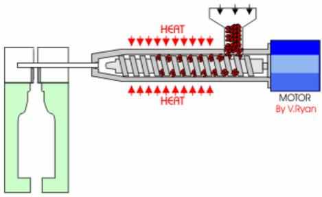
Blow moulding a shape is a common industrial process. The example shown below is of the production of a plastic bottle. The plastics normally used in this process are; polythene, PVC and polypropylene.
