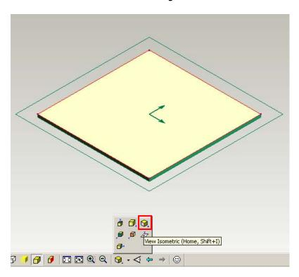
13. Next select the 'extrude icon' and then complete the extrude pop up window. Enter a feature name of 'Box sides' then enter a 'distance of 50mm', then make sure the 'above work plane' box is ticked. Then press the 'ok' button. Now press the 'save' button. Note: our original sides were 70mm high but most pupils cut there tops at 50mm. If you made your bottom and top slightly different you will have to enter a different dimension now.
