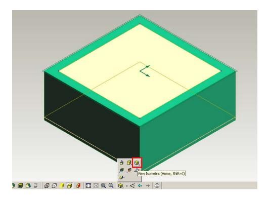
21. We have previously extruded material by adding it on to our box. We will now remove material to create the inside of our box. Now click on the 'extrude' icon and change the 'feature name' to inside box, select 'subtract material', enter a 'distance of 50mm' and select 'below workplane'. Then click on the 'ok' button.
