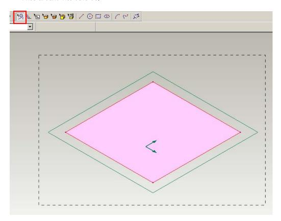
7. Now click on the 'extrude' icon below, then enter a feature name of 'plywood base', a 'distance of 3mm', ensure you select 'below work plane' and make sure the 'add material box' is select. Then click on 'ok' and your box will be extruded, now click on the 'save' button to save your work. This is shown in the image below.
