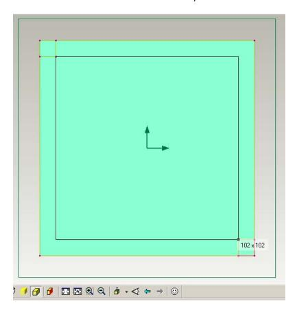
32. Next select the 'select lines' tool and click on the two small guide square and 'delete' each line. Then still using the 'select lines' tool draw a square around the outside of the smaller square to select the square. Ensure you delete all the guidelines you will no you have because your centre square will flash up with a colour like below:-
