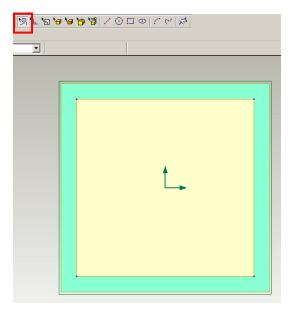
33. Now click on the 'extrude' icon and enter in the below information. Feature name 'inside lid', select 'subtract material', select a 'distance of 17mm', and select the 'below workplane' option, then press 'ok' Now press 'save' Then press the 'tumble icon' to see your box rotate, then click on the 'tumble icon' to stop your box moving.
