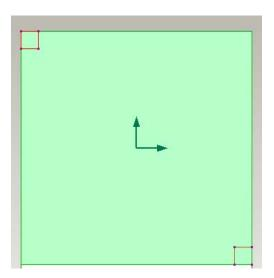
31. Now pick the 'rectangle' icon again and draw a 102mm x 102mm square from the bottom corner of the top square to the top corner of the bottom square like the image below! The rectangle tool will automatically lock on to each square. Note: these are the internal dimensions of our square box.
