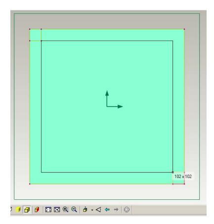
19. Next select the 'select lines' tool and click on the two small guide square and 'delete' each line. Then still using the 'select lines' tool draw a square around the outside of the smaller square to select the square. Ensure you delete all the guidelines you will no you have because your centre square will flash up with a colour like below:-
